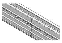
Symmetrically apply two self-tapping screws ST6.3\*22 in each side
