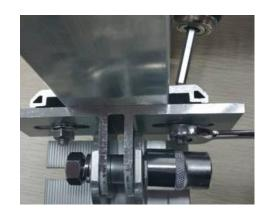
Recommended Torque for M8 bolt is 18-20Nm
