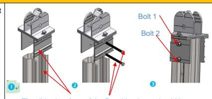
The ribbed surface of the Post Head cap should be facing the same direction as the opening direction of the post and the bolt head
