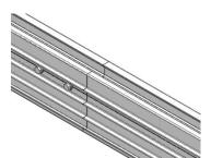
Insert the other TR-Rail onto the Splice.
