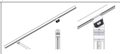
Connect the Tube Support II of the Pre-assembled Support and Post Brace with M12 hexagonal bolts and nuts and lightly fasten the nuts by hand.
