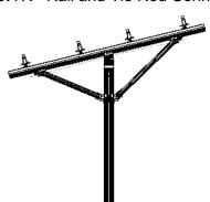
Step 2: Top and side Post Brace installation
