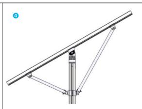
If the second Tube Support II is unable to be installed due to ramming deviation, refer to the following operations to adjust the orientation of the Post Head.
