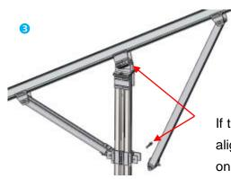
If the bolt holes are not aligned, adjust the bolts on the corrugated H Joint, then fasten it after installing the Tube.
