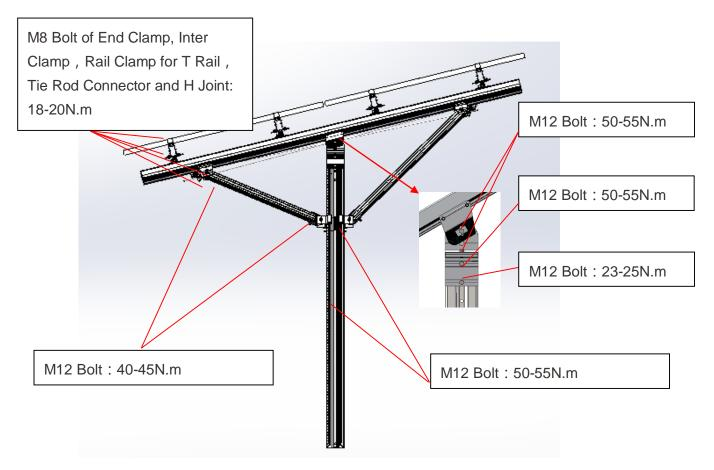
Note: Do not fasten bolts tightly until each component is adjusted properly. Repeated fastening or unlocking will result in bolt galling / deadlock.
